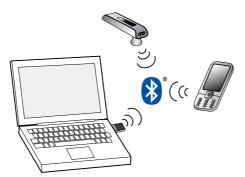
Figure 78: Jabra GO headset paired with both a mobile phone and the Jabra LINK 350 USB Bluetooth® Adapter
